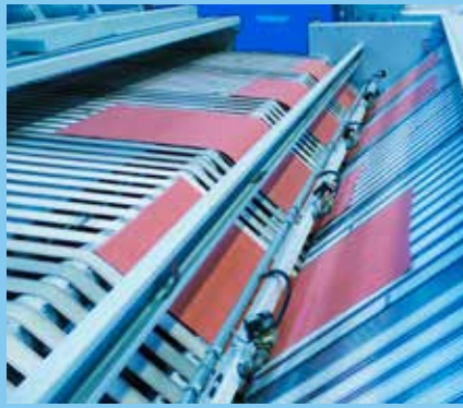
Lateral folds in multiple lanes. Airblast pipes to mark the fold is an optional feature typically used for starched linen
